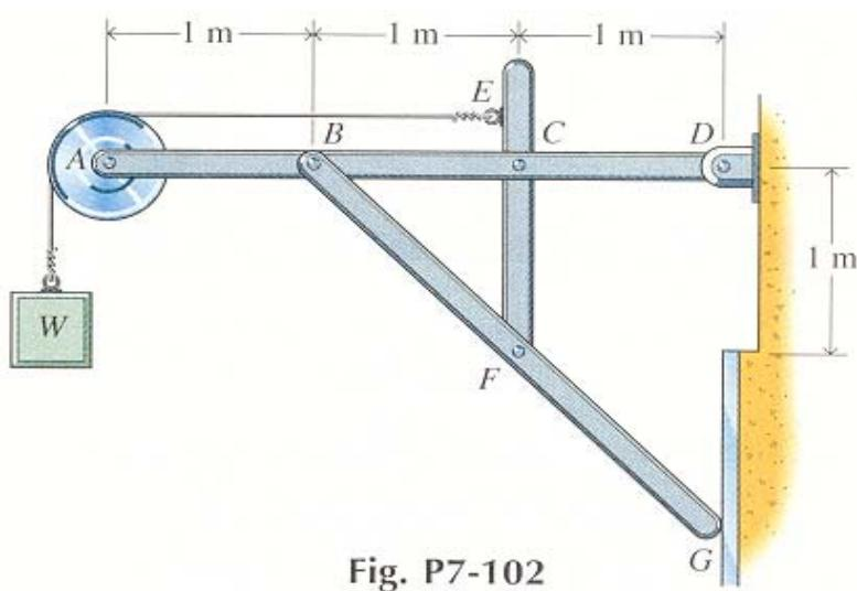
A cable is attached to the structure at *E*, passes around the 0.8 m diameter, frictionless pulley at *A*, and then is attached to a 1000 N weight *W*. Determine all forces acting on member *ABCD*.
