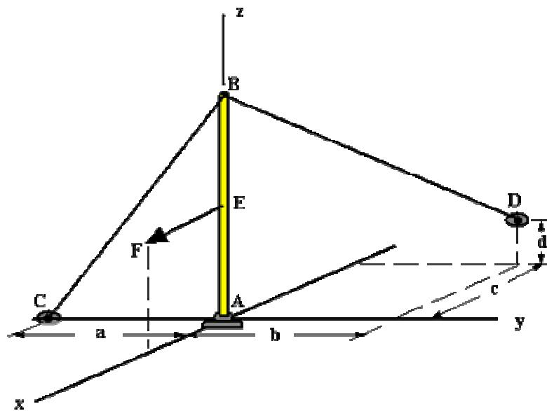
The boom AB of length  $L$  is supported by a ball-&-socket at A and two cables BC and BD. Calculate the cable tensions and the reaction at A due to the force  $F$  applied at the midpoint E of the boom.
