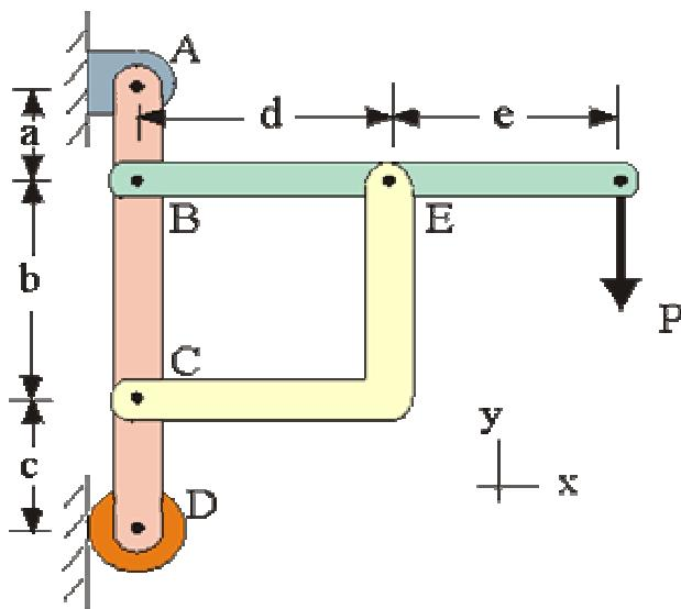
Determine the horizontal and vertical components of pin forces at A, B, C and D on member ABCD.
