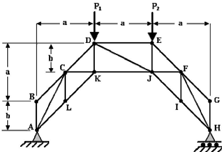
Solve for the forces acting in members DE, DJ, and KJ of the truss and indicate whether they are in tension, (T) or compression, (C).
