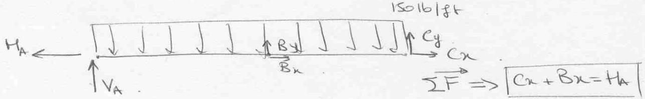
$$\begin{aligned} \sum M_A &= 0 = .5 B_y + 7 C_y - (150 \times 7) (\frac{7}{2}) \\ \Rightarrow & [5 B_y + 7 C_y = 3675] \quad \textcircled{1} \end{aligned}$$
