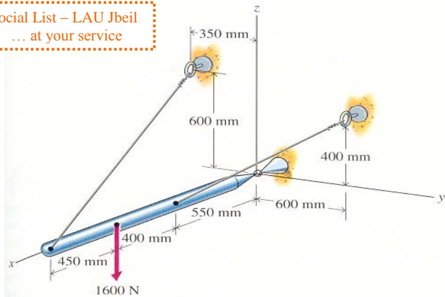
A bar is supported by a ball-and-socket joint and two cables as shown. Determine the reaction at support *A* (the ball-and-socket joint) and the tensions in the two cables.
